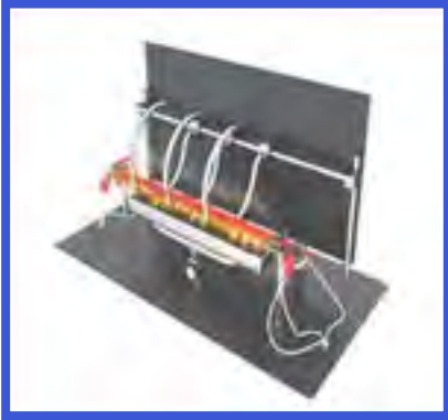
FIRE RESISTANCE (Cat. C) The cable is exposed to fire at the 950°C for 180 minutes
