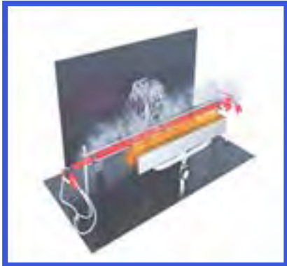
FIRE AND WATER RESISTANCE (Cat. W) The cable is exposed for 15 minutes to flame at 650°C and for additional 15 minutes to fire and water spray
