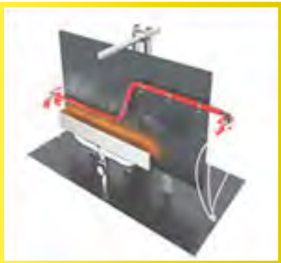
FIRE RESISTANCE WITH MECHANICAL SHOCKS (Cat. Z) The cable is mounted on a vertical panel and shocked with a steel bar for 15 minutes while submitted to the action of a flame.
